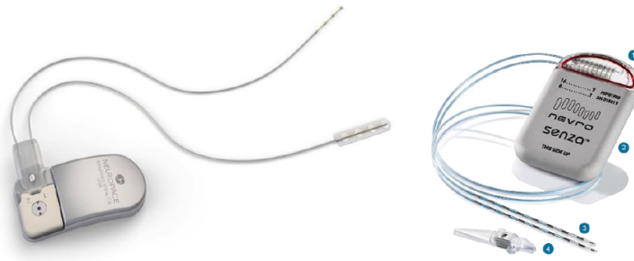
Figure 2-1: Examples of IPG-based neuromodulation devices. Left: NeuroPace RNS DBS system [1]. Right: Nevro HF10 SCS system [2].
