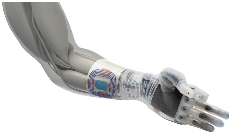
Figure 3-3: Rendering of four implants implanted in a forearm with the external transceiver cuff overlaid. (Rendering by Draper)
