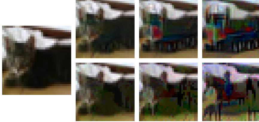
Figure 3-4: An image of a cat adversarial perturbed for different levels of distortion ( \varepsilon ). Left: the original image (i.e. \varepsilon = 0 ). Top row: \ell_2 -bounded with \varepsilon = 300, 600, 1200 (left to right). Bottom row: \ell_\infty -bounded with \varepsilon = 8, 16, 32 (left to right).
