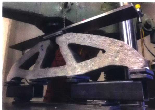
Fig.2-7 Testing of the Optimized Beam
