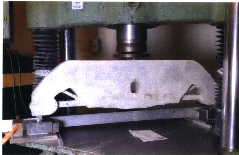
Fig.4 Experimental set-up for beam testing
