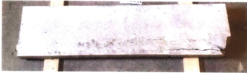
(e) Beam with full volume and traditional reinforcement
