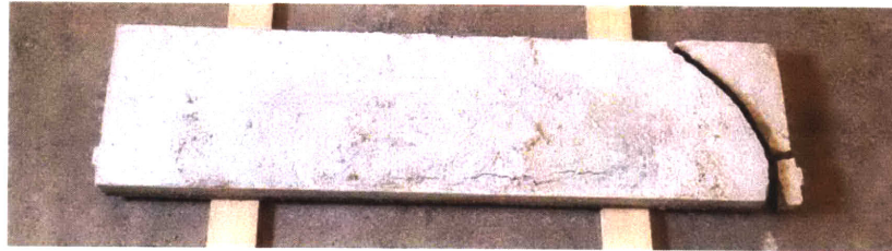
(f) Beam with full volume and optimized reinforcement
