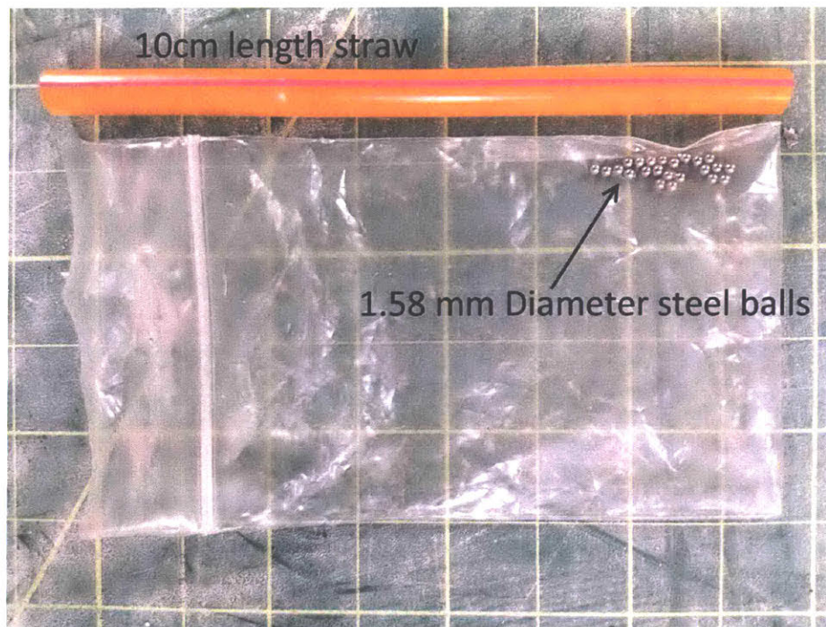
Figure A.6: To calibrate for moment magnitudes, set up all sensors, place 10cm straw vertically near center of specimen, drop ball in the straw and record the waveform. Repeat 10 or so times.
