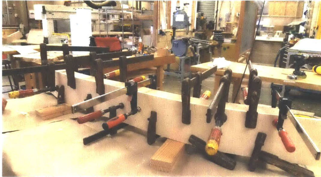
Figure 28: Three layers of \frac{1}{8} " plywood clamped to curved MDF form
