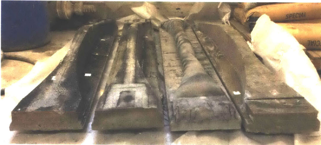
Figure 30: Final beams produced by, from left, milled foam formwork (2), fabric formwork, and bent wood formwork
