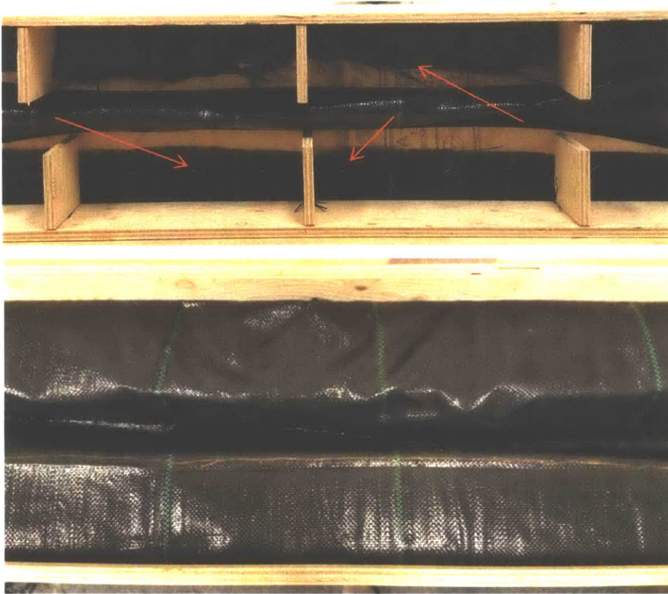
Figure 26: Fabric fabrication: (a) staples, visible from underside; (b) wrinkles in half, as seen from top
