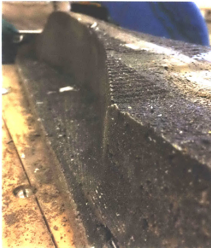
Figure 31: Texturing on the surface of the milled foam beams (Credit: Yan Liu)
