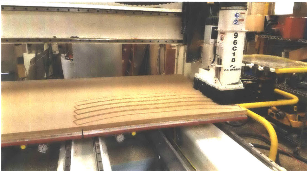
Milling of the MDF form for shaping the sides of the web.
