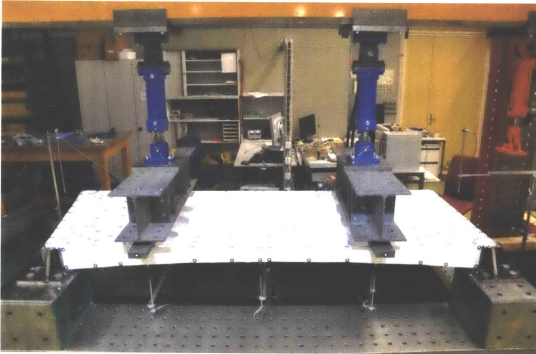
Figure 4: Complete four-point-bending experimental setup for service loading of a thin-vaulted, unreinforced concrete floor (Credit: Liew et al. 2017)
