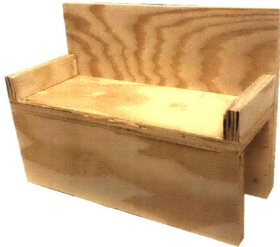
Figure 32: Complicated plywood supports made the end of each non-milled beam flat for load testing
