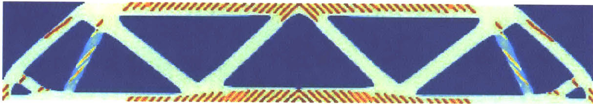
Figure 18. Full MBB Beam with Diagonal Inclusions
