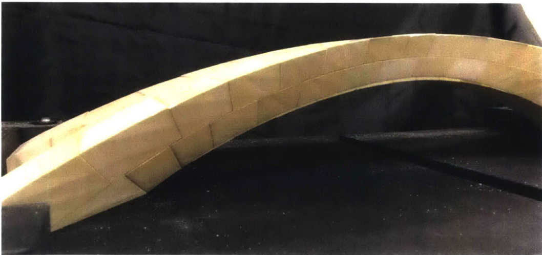
Figure 3.17 – Assembled 126 pieces with removed mold
