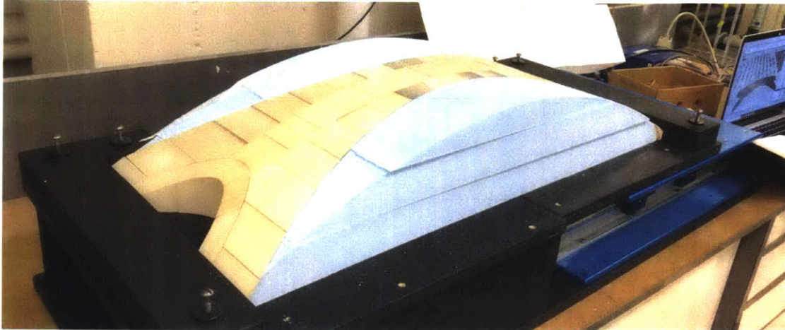
Figure 3.16 - Assembled scale model with layered formwork
