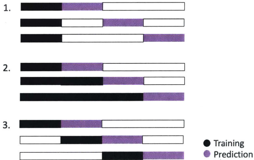
Figure 5. Different Types of Training Scenarios to Handle Concept Drift
