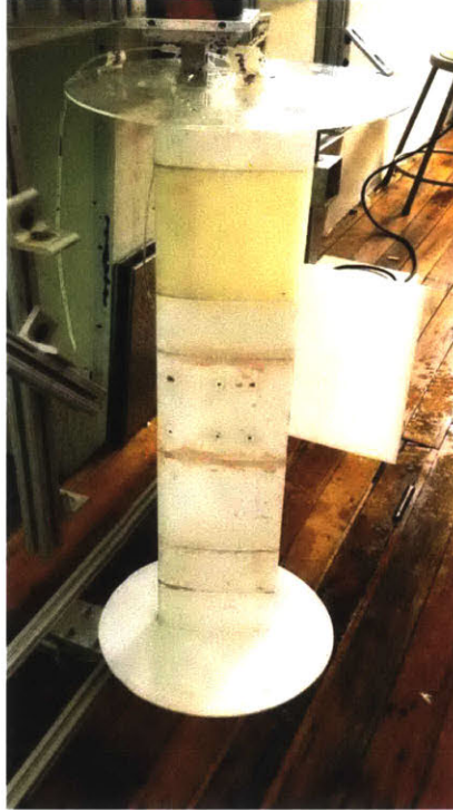
Figure 2-1: Image of NACA0018 wing in carriage. Holes in the center mark the location of the dye visualizations. Force sensors sit above and below the endcaps on the top and bottom of the wing.
