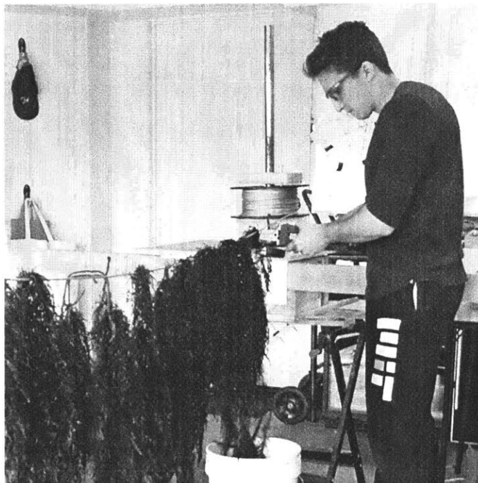
Figure 2-5: This figure shows an image of the physical test setup of the second version of the harvester. In this image, we are using a circular blade that is manually operated by my colleague, Chris, to remove the seaweed off of the line and store it in the white bucket shown in the image. The spool and the rotating mechanism can be seen at the end of the line.
