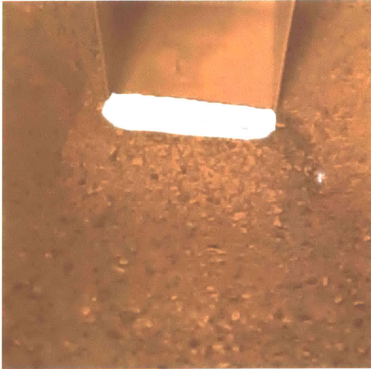
Figure 5-8: The segmentation from the U-Net model overlaid on a frame from a gaze tracking video. The segmentation is colored orange for clarity on segmented areas. The model has never seen this frame before, and it is a relatively low quality frame compared to the original images that the model was trained on.
