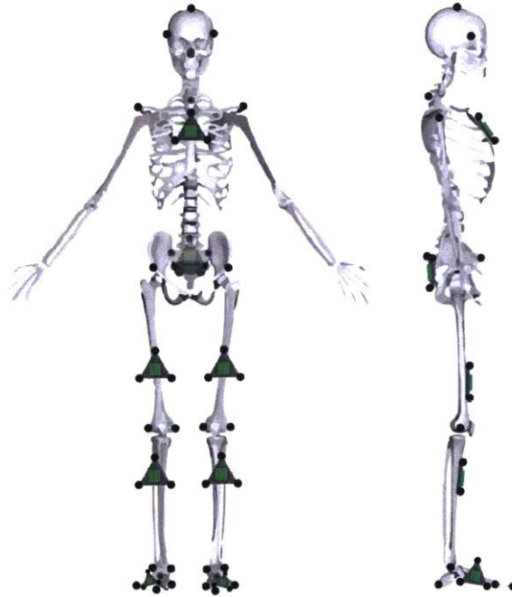
Figure 1. Placement of the reflective markers (black circles) and IMUs (green) on the subject. IMUs on the thigh and shank were not placed precisely, and location varied in the transverse plane.
