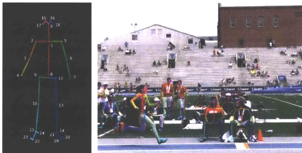
Figure 2-1: (left) The 25 signals tracked by the OpenPose demo are shown [7]. We will use the foot coordinates for this application, but the rest can be used to estimate the center of mass's location. (right) Example of how the OpenPose demo works on one of our ten long jumping videos
