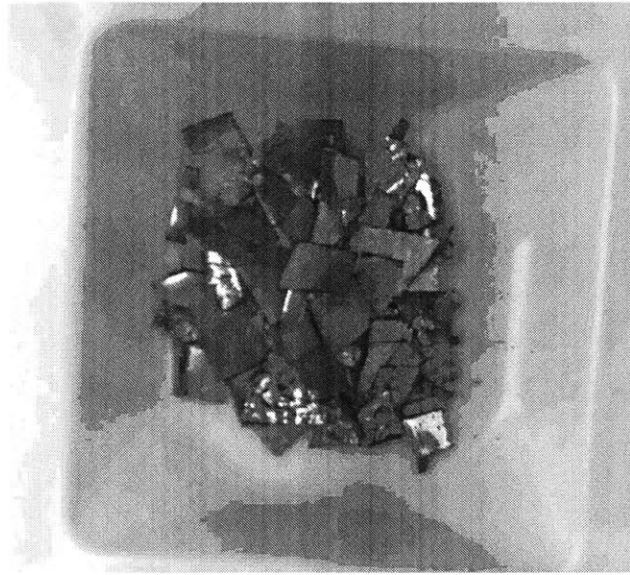
Figure 10: Flakes of Aluminum can prior to eutectic treatment
