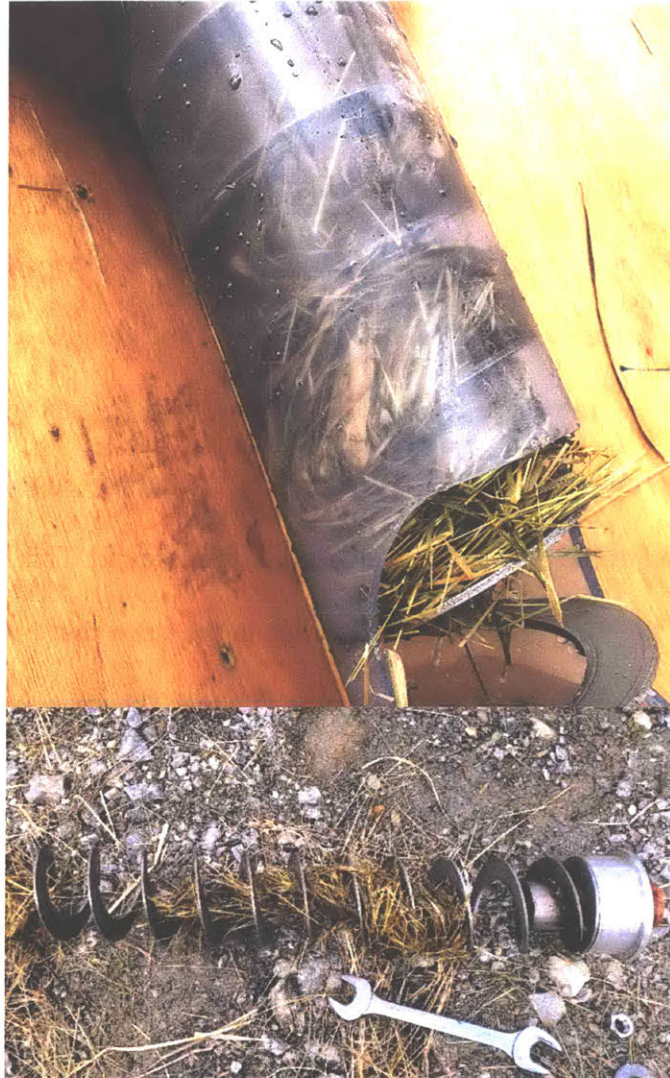
Figure 4-3: Photographs of the hay clog in the shaftless auger in the pipe (top) and outside of the pipe (bottom).
