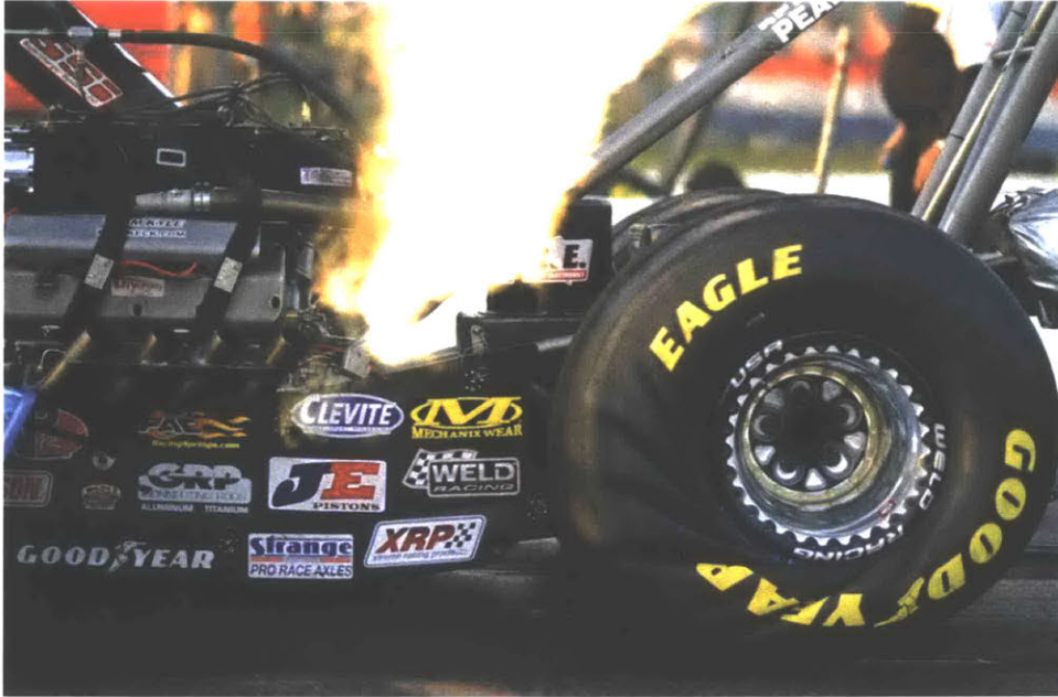
Figure 8: Dragsters' tire wrinkles are an example of extremely high slip ratio.
