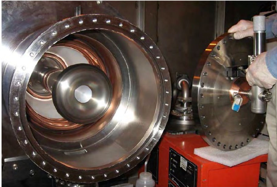
Figure 5-4: Interior structure of the Pierce type electron gun. The gun cathode is opened up for installation. The anode is attached to the flange on the right. Photo credit: Jason Hummelt [19].
