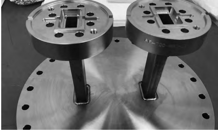
Figure 3-14: Photo of the welded SST waveguides onto the 10-inch top flange.
