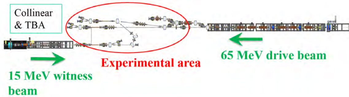
Figure 3-1: Overall layout of the AWA facility, with the 65 MeV drive electron beam line, and the 15 MeV witness electron beam line.
