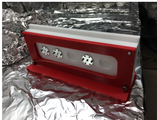
Figure 5-10: Fiber mirror assembly and storage stage. Each fiber mirror is glued to an aluminum adapter. The aluminum adapter has 0-80 through holes, which can be used to secure spare fibers, as in this picture, or to attach the fiber to an adapter that is glued to a PZT (as shown in Fig. 5-9a).
