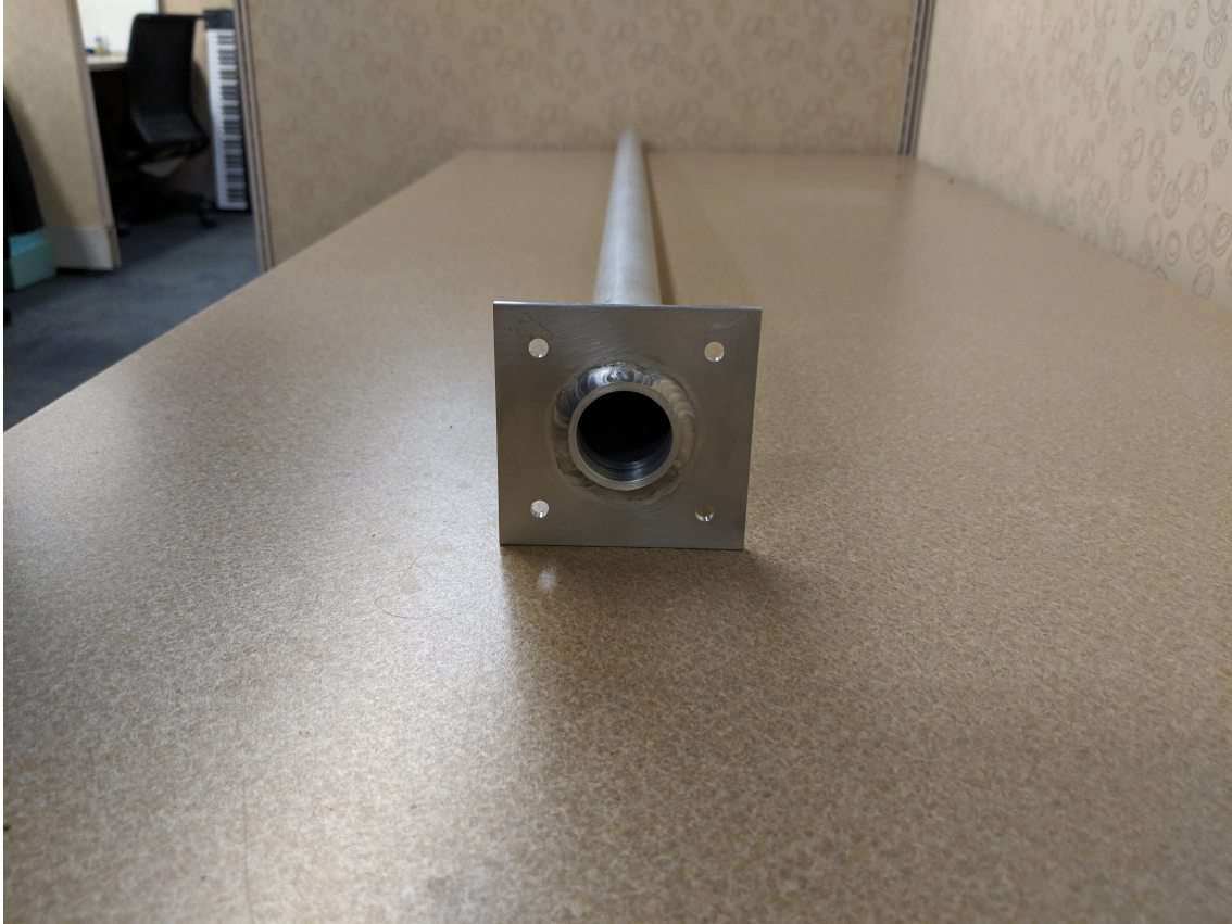
Figure 3-7: Barrier tube for the MGEP. This tube is designed to act as a stationary buffer between the control rod and the graphite of the fuel channel it is inserted into, to prevent wear on the inner channel and potential contamination of the pile.
