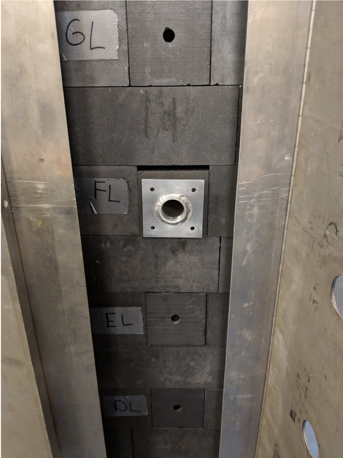
Figure 3-8: The barrier tube for the MGEP inserted into a detector channel on the East face of the pile.
