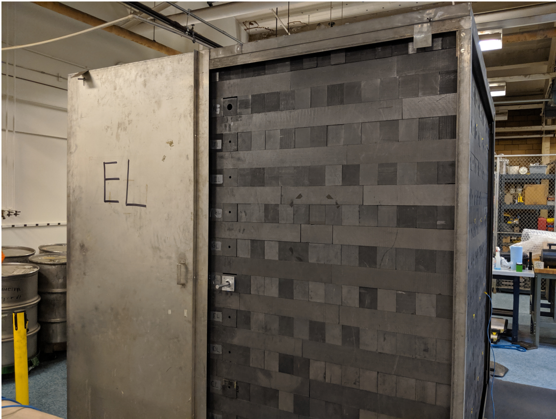
Figure 3-10: A picture showing the control rod fully inserted into the MGEP's East face, in the central detector channel which penetrates half the length of the pile.
