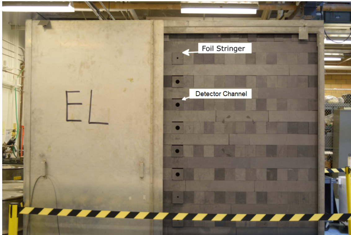
Figure 2-3: The East face of the MGEF. This picture shows the upper segment of the lattice on the East face of the pile. The detector channels as well as the foil stringer channels can be seen. The channels only run half the length of the pile [6].
