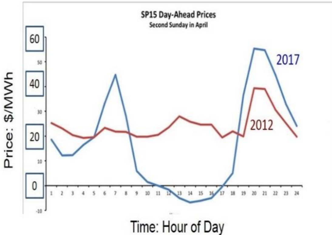
Figure 1-1: The price of electricity in California on a spring day in 2012 and 2017. Between these days, a large amount of solar generating capacity was added, leading to the price crash at midday in 2017. [1]
