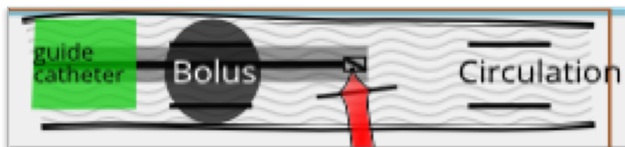
Figure 2-1: Diagram of Bolus Injection Entering the Circulation. The bolus injected travels through the guide catheter and exits at the end of it to enter the circulation. The bolus travels through, initially displacing the entire circulation and mixes fully with the circulation flow as the circulation returns.
