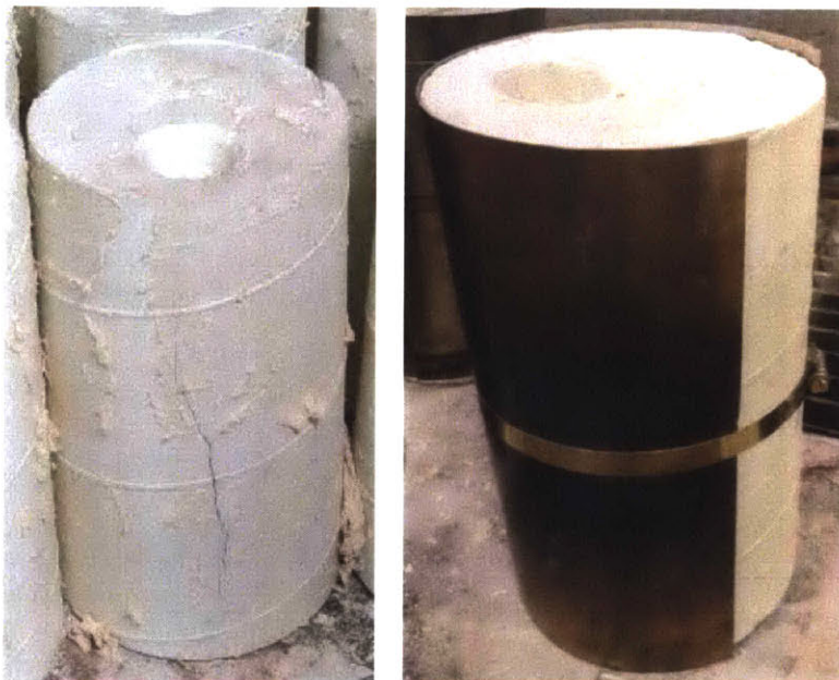
Figure 26 Mold Cracking Mitigation
