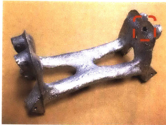
Figure 42 Punctured Hole in Optimized Connection
