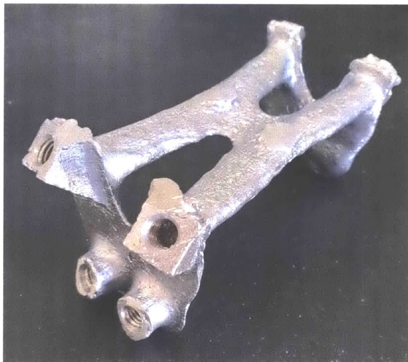
Figure 34 Original Eight Holes for Attaching Connection into Testing Frame
