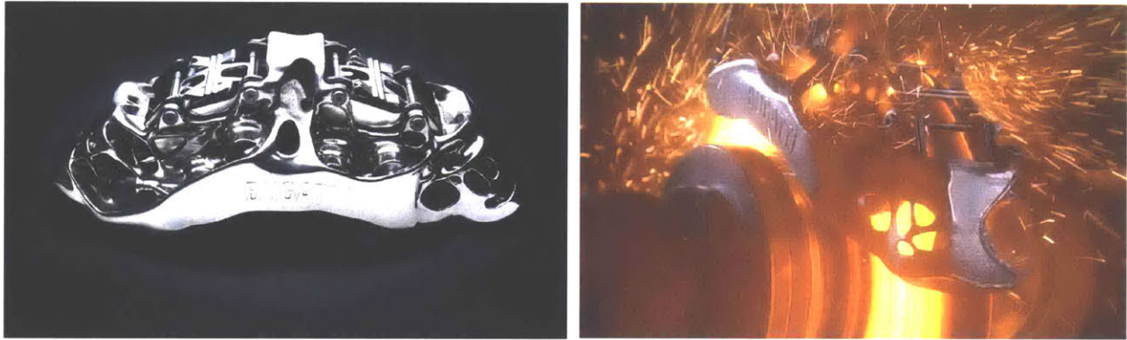
Figure 9 Bugatti Brake Caliper with Pistons and Pads Fabricated & Tested (Molsheim and Wolfsburg 2018)
