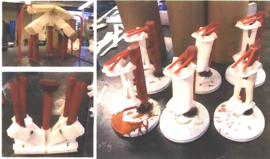
Figure 24 Investment Casting Wax Preparation
