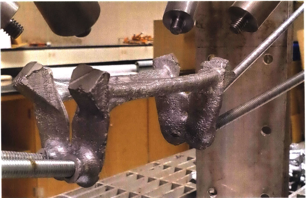
Figure 35 Fitting the Specimen into the Testing Frame
