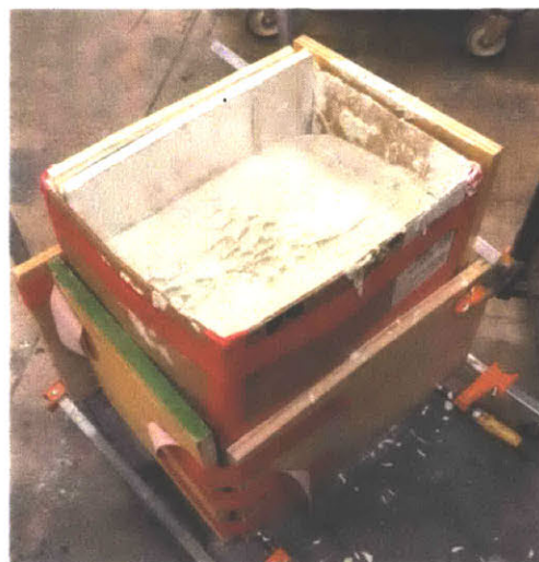
Figure 25 Glass-Cast Investment Mixed and Poured before Placing in Furnace
