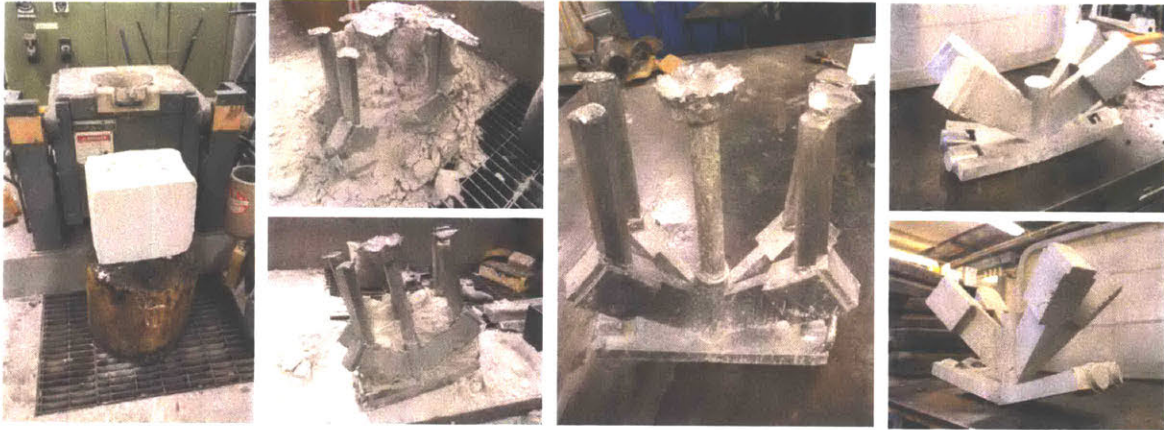
Figure 27 Casting Post - Processing: Part Extraction
