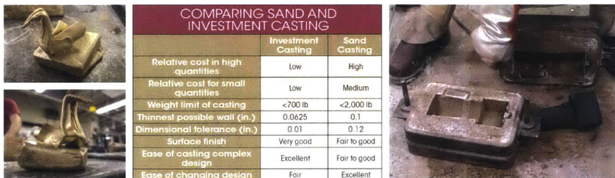
Figure 12 Investment vs. Sand Casting Performance Comparison (Done 2016)
