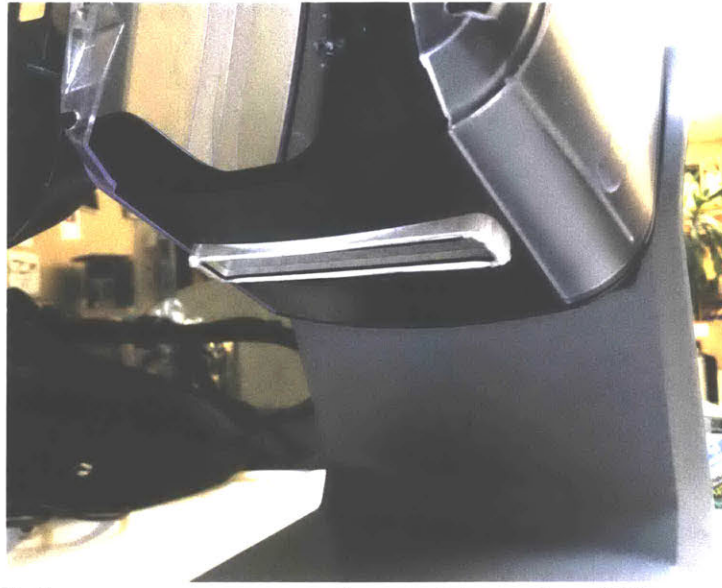
Figure 3.8: Pressure sensor wrapped around inner rim of dispenser opening.
