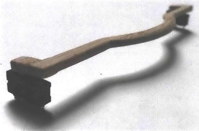
Figure 3.11: Photo of final mechanical lever – bowed out geometry chosen
