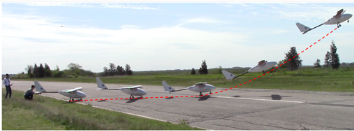
Fig. 9 In the Large Propeller configuration with 25° flaps, the vehicle demonstrates a takeoff roll of 2.0–2.5 vehicle lengths, and a maximum climb-out angle of 21 deg.
