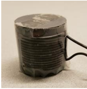
Fig. 10: Prototype inductor. Vertical windows in the outer shell were added to impede the circumferential component of flux and to allow the winding terminations to leave the structure.
