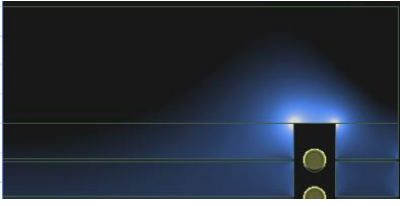
Fig. 5: Flux crowding at the end of the window leads to higher B fields (white and light blue) and thus greater core loss.
