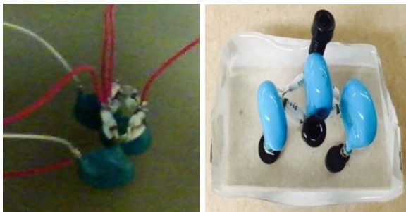
Fig. 10 Air-insulation (left) and PDMS insulation (right)
