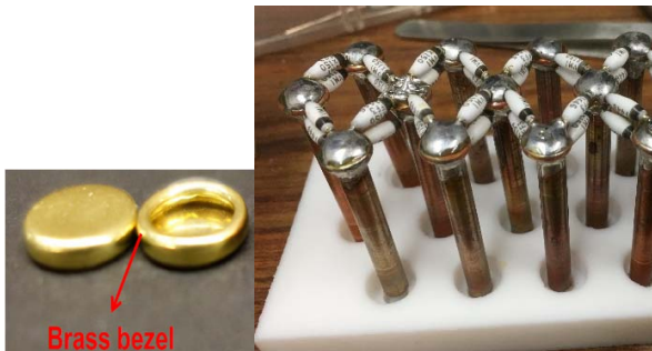
Fig. 9 Air-insulation (left) and PDMS insulation (right)
