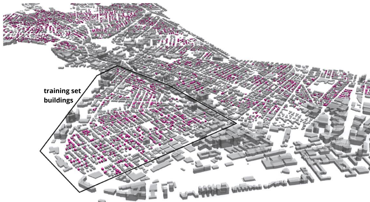
Figure 2-2: 3D view of the urban building energy model for the city of Cambridge (Sokol et al. 2017). The outlined building subset was used to train models that could then effectively simulate all neighborhoods.
