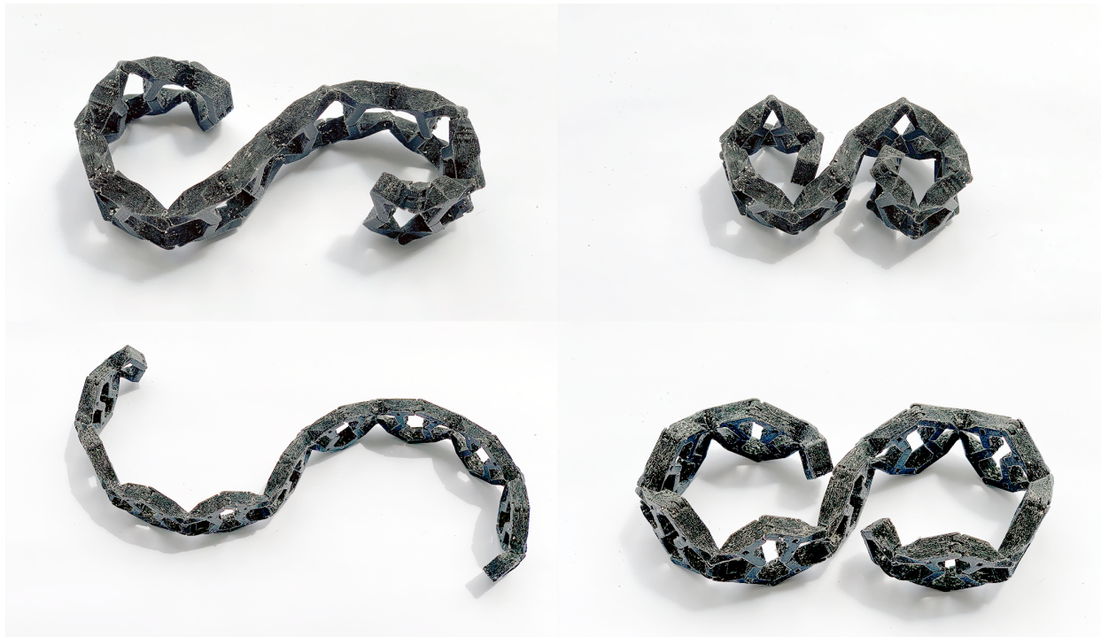
Figure 39. The top two images are the 3DP result, the bottom two images shows the assemble result.
