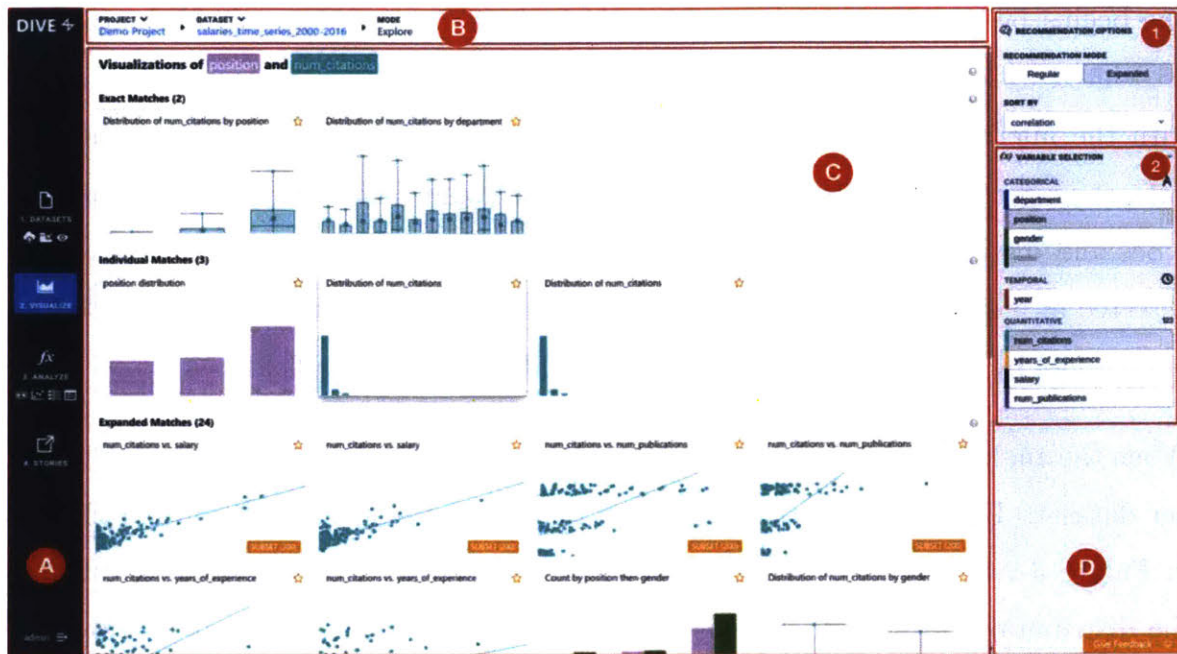
Figure 3-2: The DIVE user interface. The left navigation bar labeled (A) is used to navigate between modes and modify project properties. The top navigation bar labeled (B) marks the current user state (project, dataset, and mode) and lets users switch projects or datasets. The main pane labeled (C) displays the main results of the mode. The right selection menu (D) lets users change mode-specific parameters (D1) or selecting fields (D2). All other modes in DIVE follow this hierarchical four-section layout, though some modes do not include a selection menu (D).
