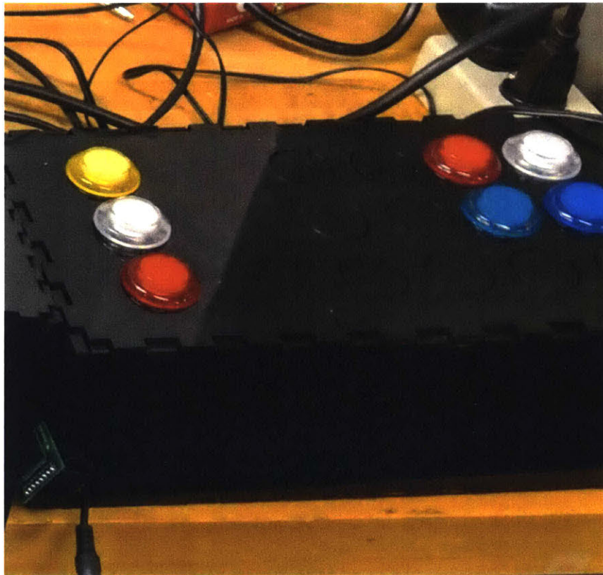
Figure 38: Shielded control box with arcade style buttons.
