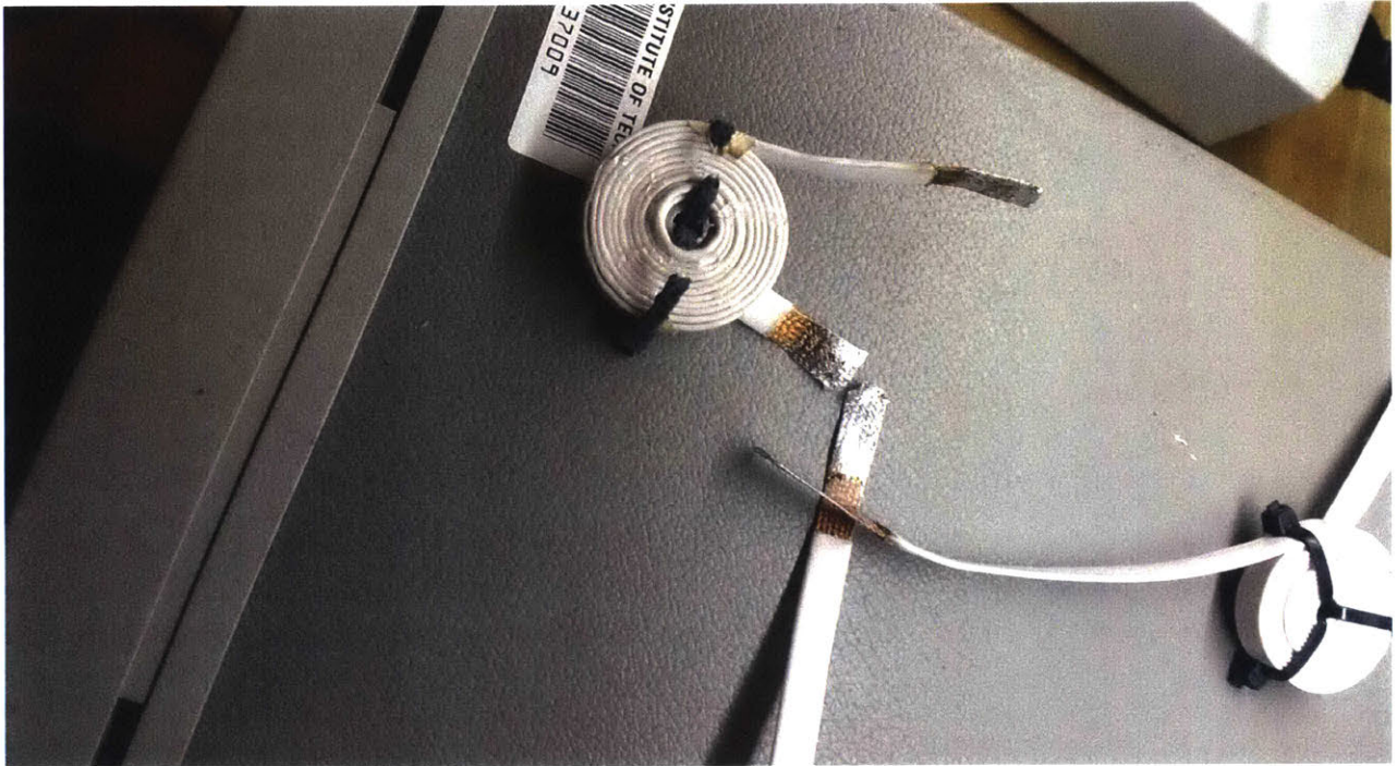
Figure 25: Initial 30mm Litz wire test coils.
