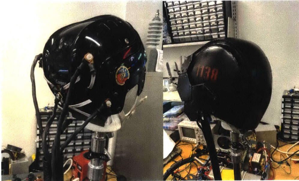
Figure 36: Wearable array with isolation hood for dark adaptation.
