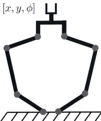
Figure 2-4: A closed kinematic chain manipulator. For simplicity, we can assume that the first three joints of each sub-chain are actuated.
