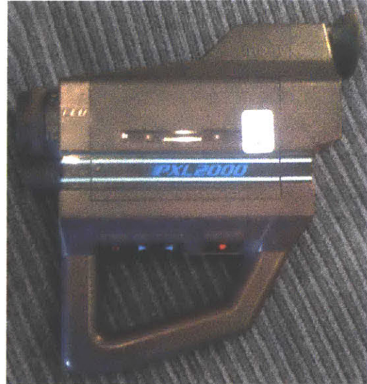
Figure 15 – The Fisher-Price PXL-2000 “pixelvision” camera. (Photo by Joe Lillibridge, 2008. CC BY-SA 2.0)
