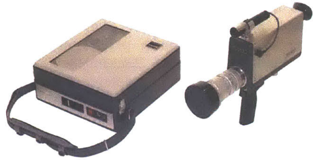
Figure 13 – A Sony AV-3400 Portapak camera system. (Photo by Wikipedia user Mwf95, 2005. CC BY-SA 4.0)
