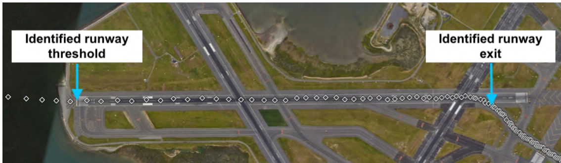
Figure 3-4: Example of the runway threshold and runway exit identified for a landing flight at Boston Logan International airport (KBOS)
