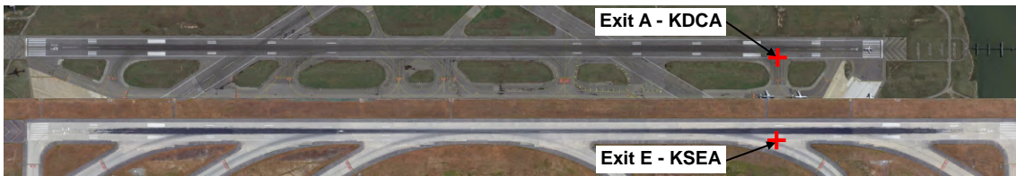
Figure 5-7: Example of similarly located high-speed (30°) and right-angle (90°) exits
