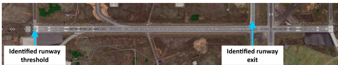
Figure 7-4: Example of the runway threshold and runway exit identified for a landing flight at Keflavík airport (BIKF)
