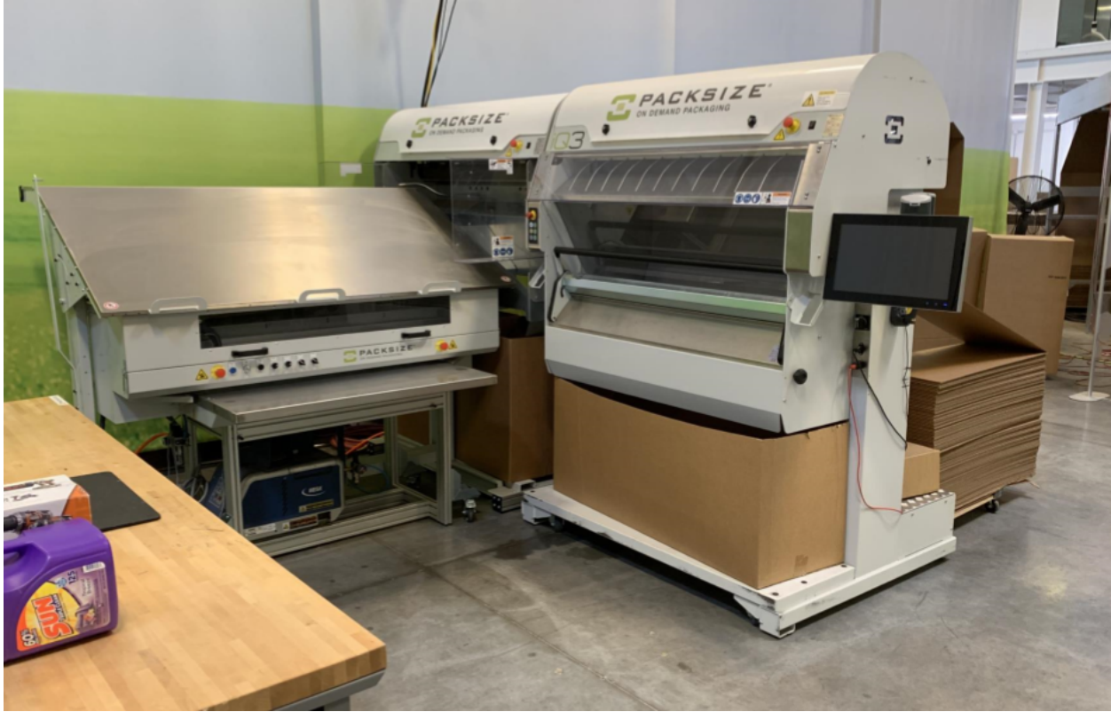
Figure 10. Packsize Custom Box Maker [Source: Packsize]
