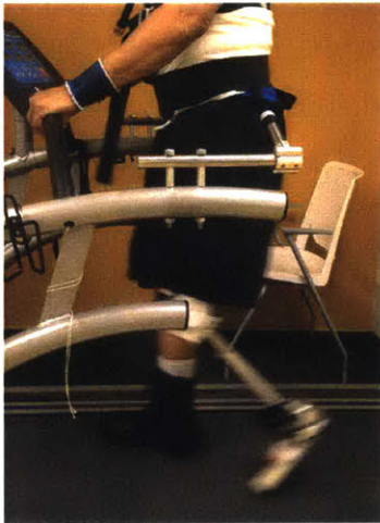
Figure 4-3: Treadmill study has shown that mean peak knee flexion angle decreased as the damping coefficient increased. The subjects walked at a constant speed on a treadmill with different damping conditions. All subjects were able to achieve knee flexion in the able-bodied range (gray band shows one standard deviation for able-bodied subjects). The no-damping condition resulted in hyperflexion during swing phase for all of the subjects. The error bars show the standard deviation of the measurements.
