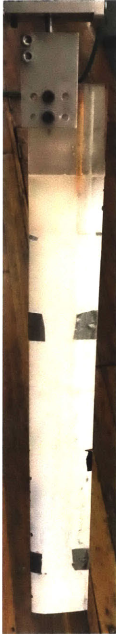
Figure 2-4: Fabricated wing for dye visualization. The wing pieces were printed on a Form II printer, assembled and sanded, and sprayed with waterproof paint to be visible underwater.
