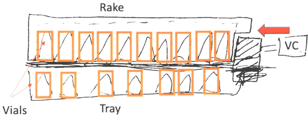
Figure 4-15: Front view sketch of a rake holding vials sitting above a tray holding vials. The back square on the right side represents a pushing block connected to a voice coil. Note: This is a modified image of the initial drawing created during the first month of prototyping. Although the outline of the sketch remains the same, an orange box has been inserted to represent a vial in traditional rectangular form. The red arrow represents the direction of travel of the biasing block. Furthermore, typeface has been placed on top of traditional handwriting for the sake of legibility
