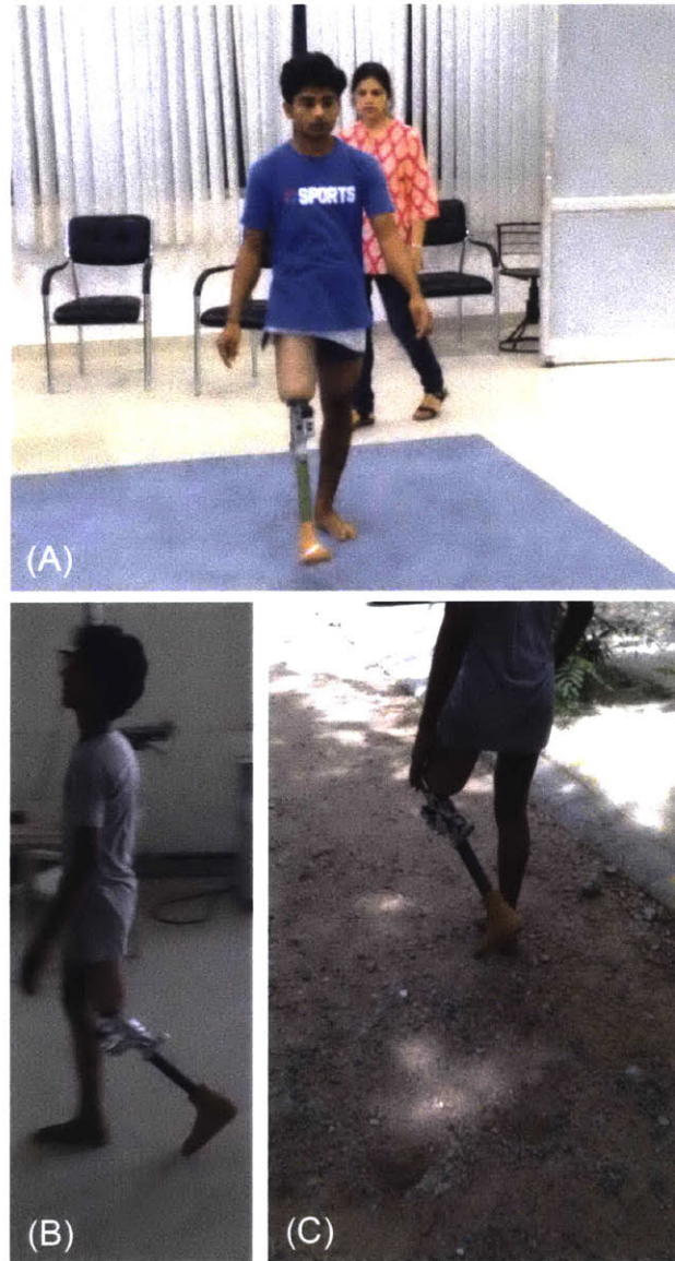
Figure 3-5: Preliminary field evaluation. (A) Subject 1 using the prototype for the 2-minute walk test. (B) Subject 2 during the 2-minute walk test, late stance flexion of up to 40 degrees can be seen. (C) Subject 2 walking comfortably outdoors on a relatively flat, muddy terrain.
