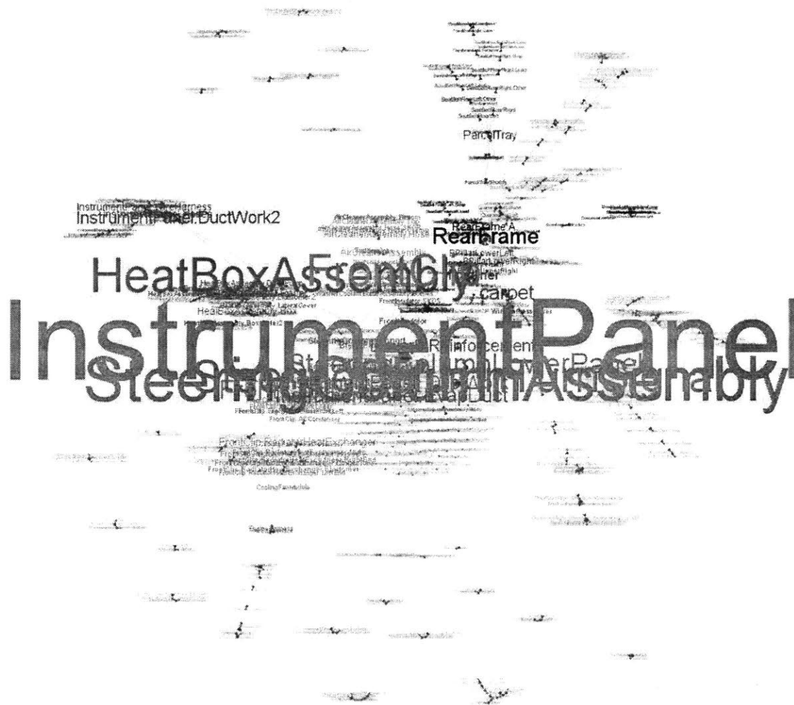
Figure 1.7 Parts and assemblies arranged by connection constraints using data adapted from [27]
