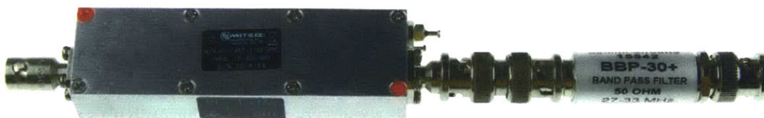
Figure 2-10: The NMR signal was amplified by a low noise preamplifier and sent through a band-pass filter.
