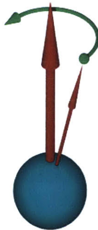
Figure 1-1: The nuclear magnetic moment, represented by small arrow, will precess about an external magnetic field, represented by the large arrow. Figure reproduced from [10].
