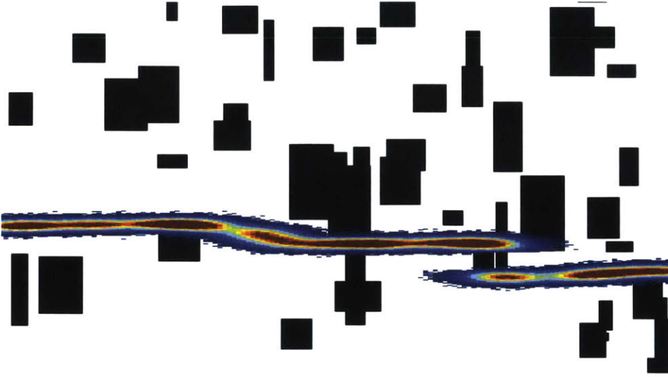
Figure 3-5: Example simulations where the AUV must traverse a 50 obstacle field. The color map denotes the frequency of AUV location over 10,000 simulations.
