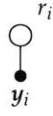
Figure 3-6: Sparse MRF model for a single beam: y_i is the measurement (quantized acoustic intensity for the i^{\text{th}} beam, over the range [r_{\min}, r_{\max}] ), and r_i is the unknown state - the range to the scatterer. A sonar scan can be considered as up to B of these models.
