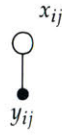
Figure 3-4: Dense MRF model for a single site (i, j) - y_{ij} is the measurement (quantized acoustic intensity at r_i, \alpha_j ), and x_{ij} is the unknown state (e.g. “background” and “target” for x_{ij} = 0, 1 , respectively). A sonar scan can be treated as R \times B of these models, assumed independent.
