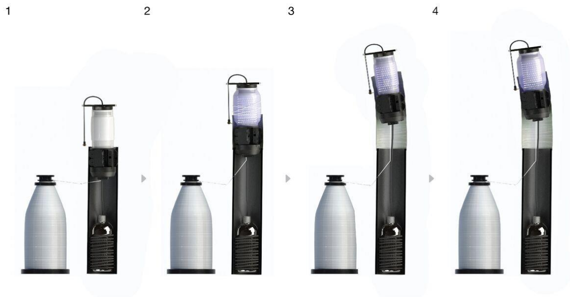
Fig. S1. System overview. (1)-(4) shows the sequence for the construction of a single segment of the composite tube with a single robot. (1) is the initial setup of the system, consisting of a spool of fiberglass thread, steel base, resin reservoir, and a single robot. The robot is tethered to the base via the black cable, which provides resin, electrical power, and communication with the resin pump. (2) shows an inflated robot, with UV LEDs turned on, as it winds a single segment. (3) shows a deflated (and hence delaminated) robot, after completing a third segment, it has driven up and tilted itself to curve the next segment of the composite tube. (4) Shows the robot inflated once more, with an overlap over the previous segment, and is ready to wind another segment.
