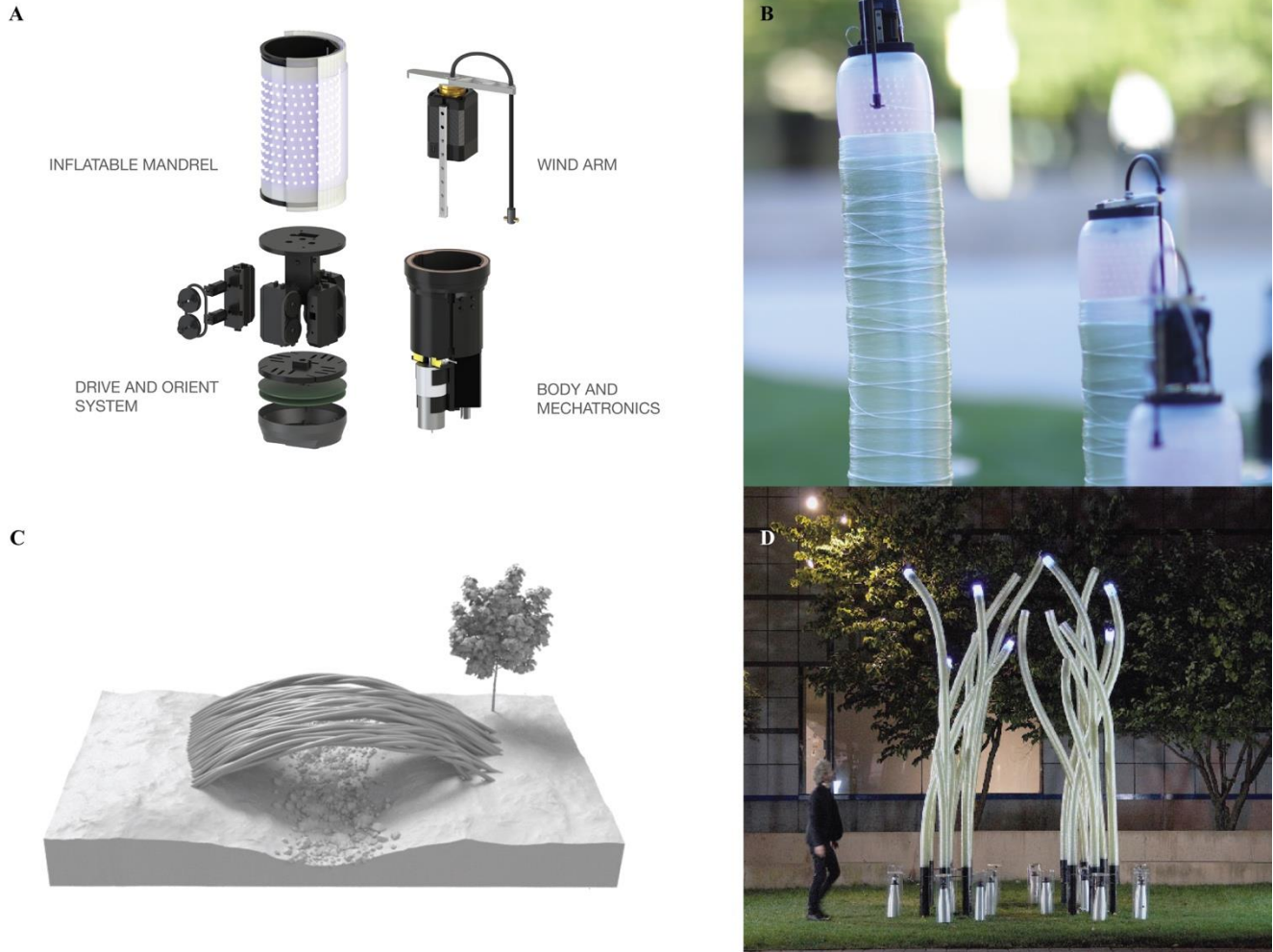
Fig. 1. (A) Each Fiberbot consists of a wind arm, a reversibly inflatable mandrel, and subsystems for navigation and control. (B) By winding fiber and photocurable resin around themselves, robots create fiber-reinforced composite tubes that they can climb and extend. (C) A possible application of the system to create a useful structure is proposed using a design flocking framework, although the spacing between tubes is narrower than can be fabricated by our current system. (D) An architectural scale print was built by 16 identical Fiberbots operating in parallel over two days.
