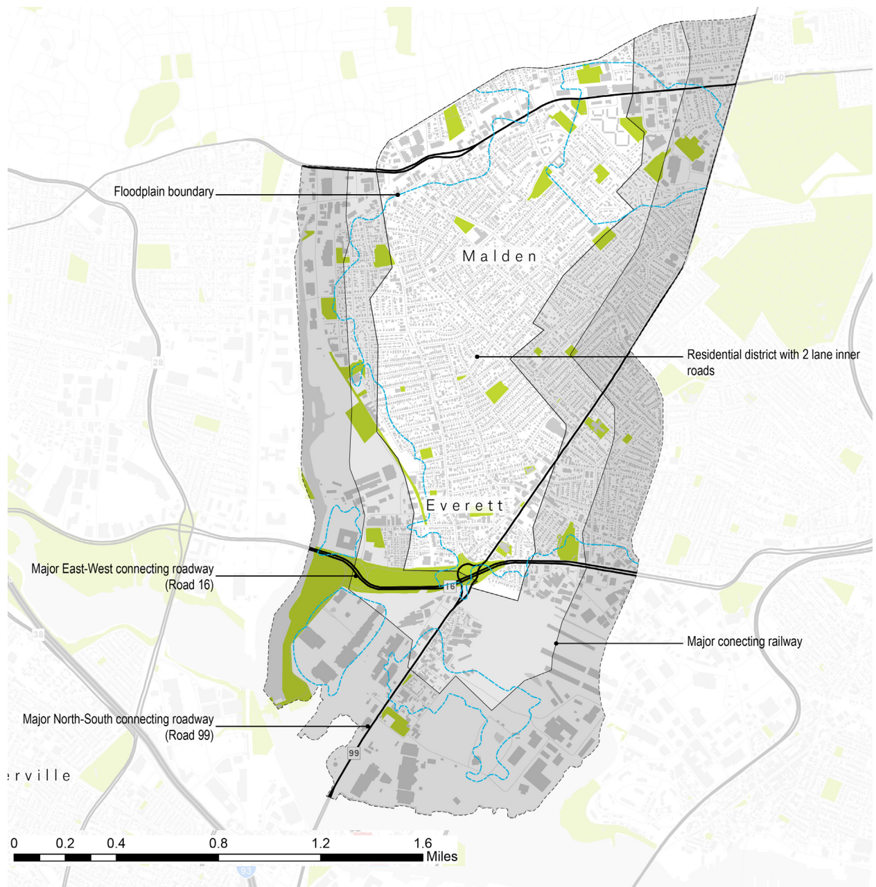
Figure 25 The Everett-Malden Resilience District Key Characteristics
