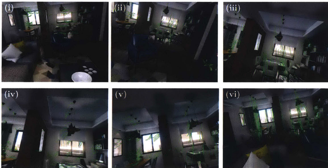
(c) Six photorealistic images generated and streamed to the drone in real time for VIO state estimation during a VIO experiment around an oval trajectory. Green lines show 0.3 seconds of history for visual features detected and tracked by the vision front end. Our simulation system generates photorealistic images at 60 Hz based on motion capture pose estimate, which are processed by the VIO system, and used in-the-loop for controlling the drone's flight.
