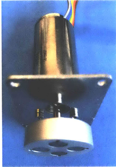
Figure A.6. The driving motor with four magnets on its shaft.
