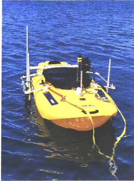
Figure 4-2: One of two Jetyak ASVs used during real-world experiments, collecting acoustic data to demonstrate the effects of range and speed on the RL of the received signal emitted from the source.
