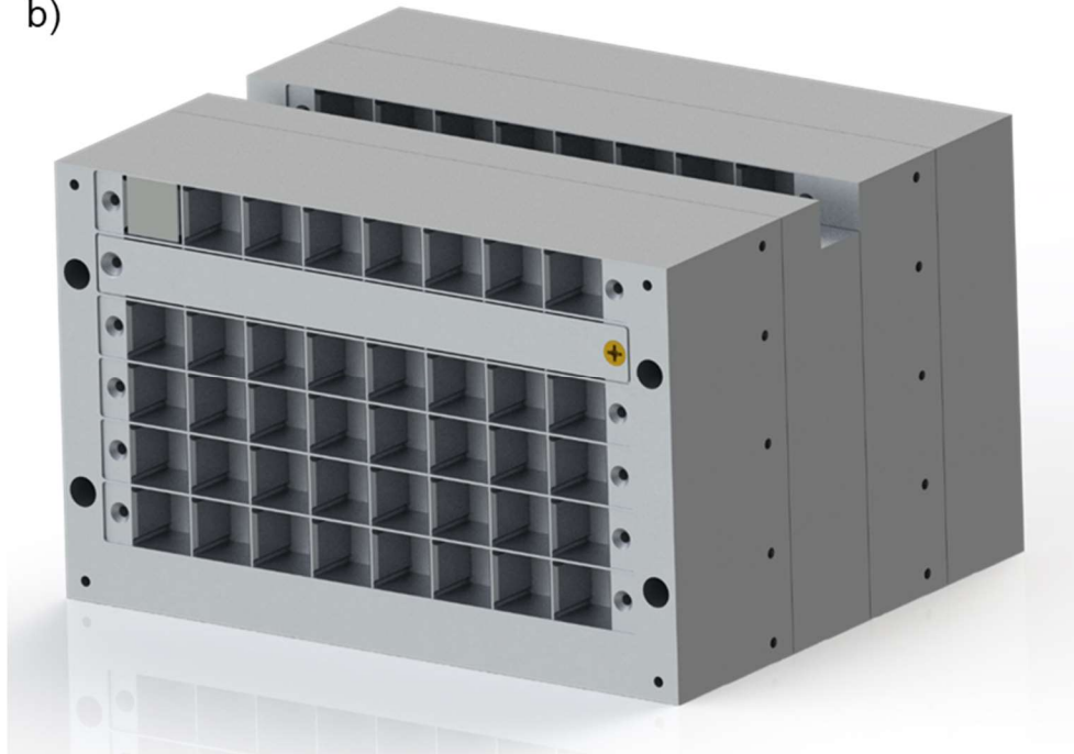
Figure 2.5. Renderings of magnet assembly. Renderings of a) a single aluminum fixture and b) all aluminum slices for the magnet assembly. For illustrative purposes, a single magnet is placed in the first row, a single row has its aluminum cover in place, and a single brass screw is fastening the cover on the right. Each square pocket has a side length of 12.7 mm.
