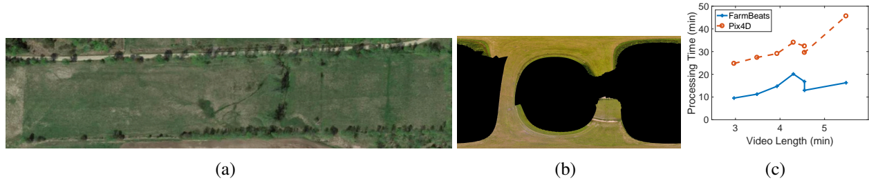
Figure 3-8: Orthomosaic Generation: (a) The Google Earth image for the farm in Figure 3-4. (b) Microsoft ICE image stitching pipeline fails to reconstruct it accurately. (c) Pix4D takes about 2.2x longer on average compared to our approach.
