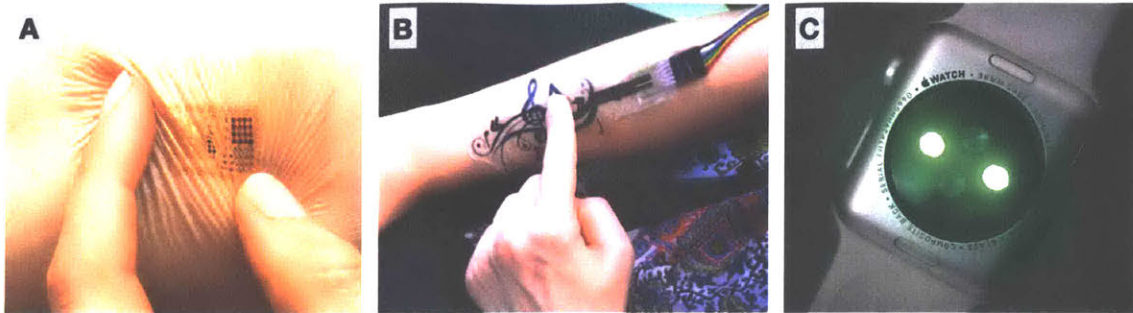
Figure 2-2: Examples of state-of-the-art wearable devices. A) Epidermal electronics: microfabricated stretchable electronics. B) iskin, an on-skin electronics using conductive ink. C) Apple watch with the green LED tuned on, which is used for measuring heartrate and blood oxygen level.
