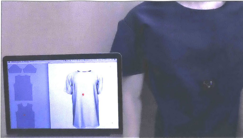
Figure 5-11: Localization of the robot on a fabric in 3D space.
