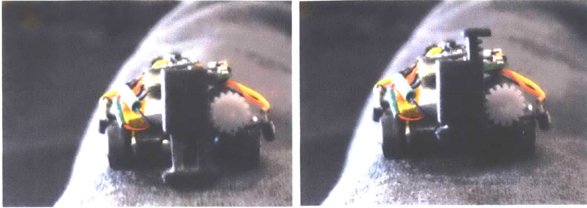
Figure 9-14: Tactile feedback application. We designed a linear actuator that can poke the skin. This tactor can go up and down to create tactile feedback.
