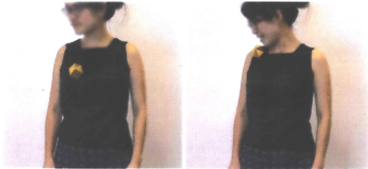
Figure 9-16: Interactive moving jewelry. Robotic brooch moves to become a shoulder microphone speaker when wearer receives a phone call.
