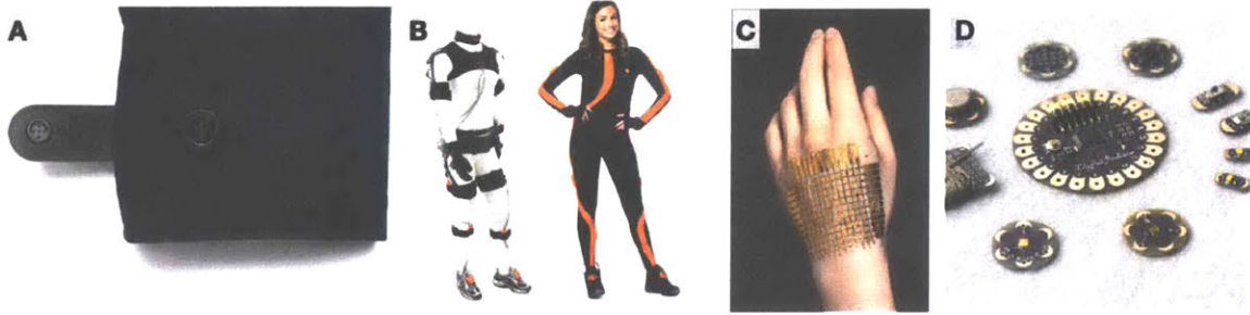
Figure 2-4: Examples of sensor suits and skins. A) Denum Jacket with capacitive sensing conductive fibers. B) Body motion capture suit from Xsens. C) Pressure sensor skin from Takao Someya's group. D) LillyPad Arduino, a kit for wearable electronics.
